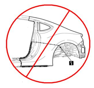
**NOTE**: The P-Cut Small Section replacement procedure may lead to one or more of the following unacceptable conditions:
